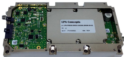
Band 7 DL (2620-2690MHz) 50Wpeak AH1 housing : 78mm x 150mm x 21mm
